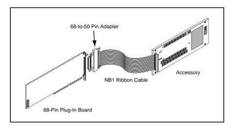
Perform the following steps to install the R6850 cable assembly:
